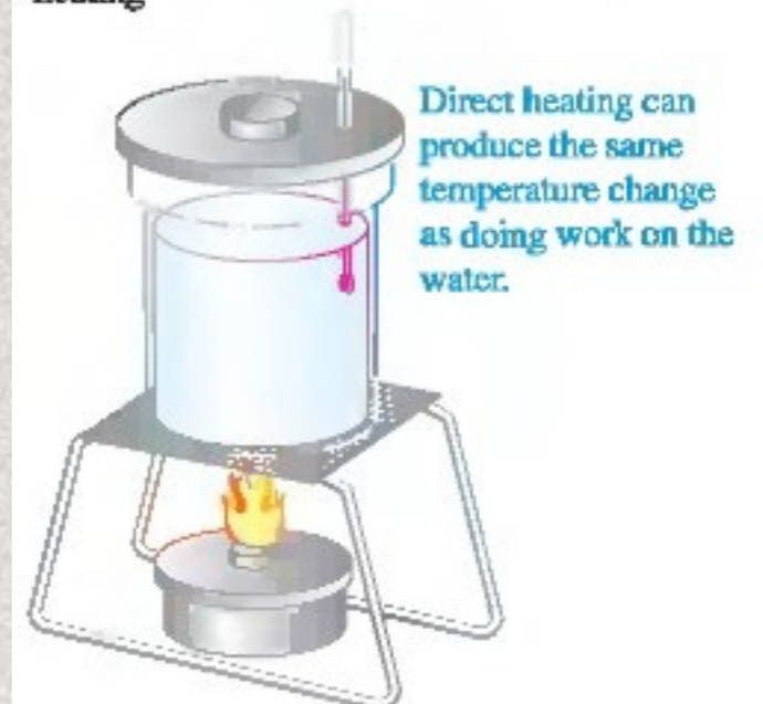
(b) Raising the temperature of water by direct heating
