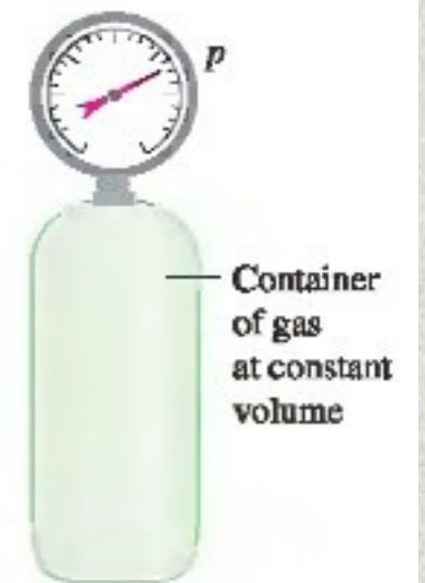
(b) Changes in temperature cause the pressure of the gas to change.
