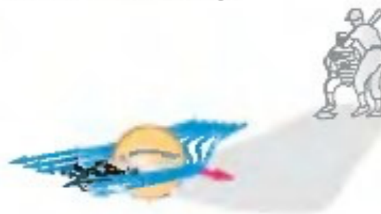
(e) Spin causing a curve ball to be deflected sideways
