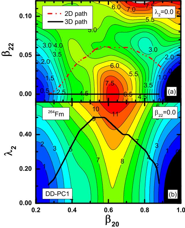
FIG. 3. Projections of the 3D dynamic path (solid curves) for the spontaneous fission of  $^{264}\text{Fm}$  on the  $(\beta_{20}, \beta_{22})$  plane for  $\lambda_2 = 0$  (a), and the  $(\beta_{20}, \lambda_2)$  plane for  $\beta_{22} = 0$  (b), calculated using the dynamic programming method. The dash-dot-dot curve denotes the 2D path computed without the inclusion of dynamic pairing correlations.
