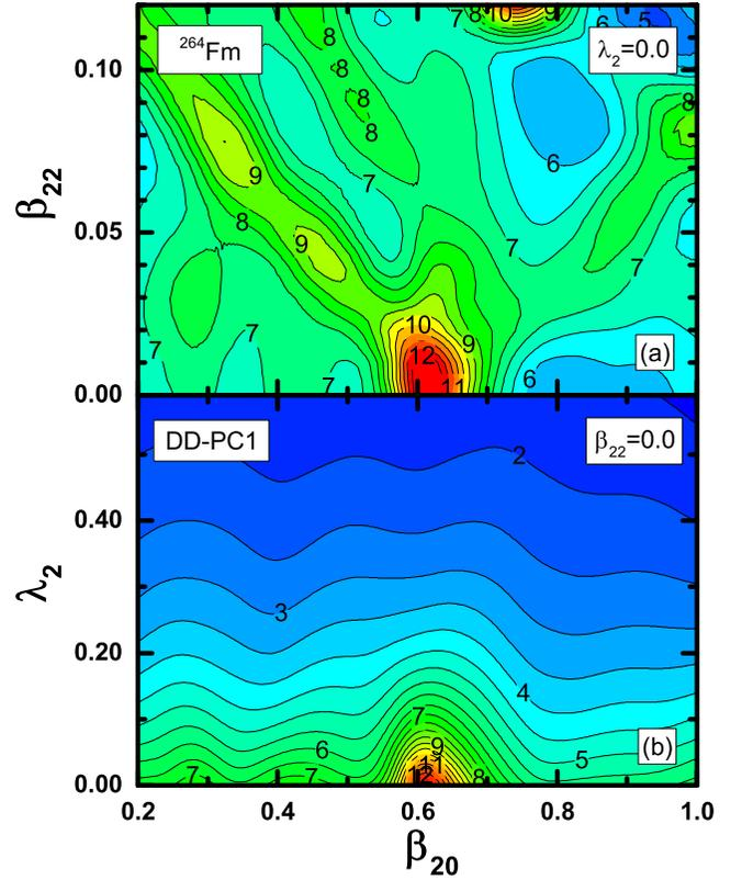
FIG. 2. Cubic root determinants of the nonperturbative-cranking inertia tensor  $|\mathcal{M}^C|^{1/3}$  (in  $10 \times \hbar^2 \text{MeV}^{-1}$ ) of  $^{264}\text{Fm}$  in the  $(\beta_{20}, \beta_{22})$  plane for  $\lambda_2 = 0$  (a), and in the  $(\beta_{20}, \lambda_2)$  plane for  $\beta_{22} = 0$  (b).
