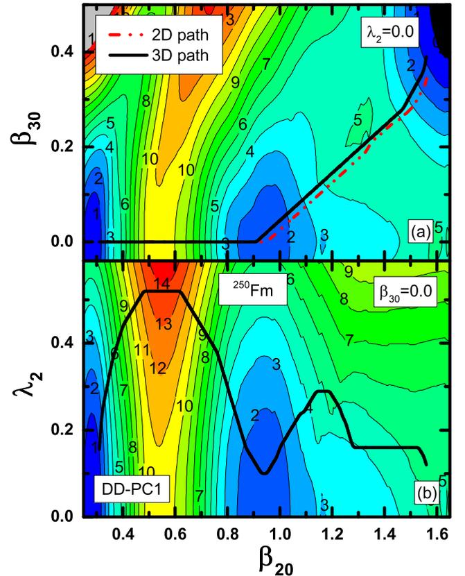
FIG. 8. Projections of the 3D dynamic fission path (solid curves) of  $^{250}\text{Fm}$  on the  $(\beta_{20}, \beta_{30})$  plane for  $\lambda_2 = 0$  (a), and the  $(\beta_{20}, \lambda_2)$  plane for  $\beta_{30} = 0$  (b). The dash-dot (red) curve denotes the 2D path computed without the inclusion of dynamic pairing correlations.
