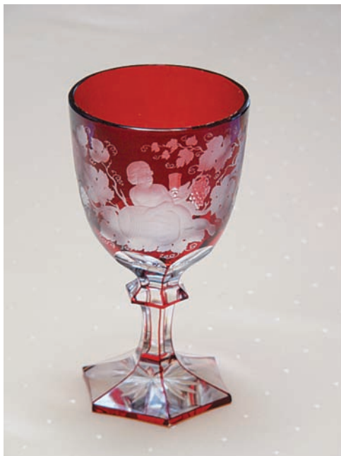
Figure 9.32 Beaker covered with gold ruby glass – a composite consisting of gold nanoparticles. Note the faint blue hue in the color, which is typical of pigments based on gold nanoparticles. (Photo: D. Vollath.)
