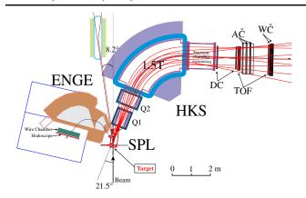
FIG. 1 (color online). Schematic figure of the E01-011 experimental setup. A newly constructed HKS and an ENGE-type splitpole spectrometer that was also used in E89-009 were used as the kaon and scattered electron spectrometers. The HKS detector package consists of drift chambers (DC), time-of-flight counters (TOF), aerogel Čerenkov (AČ) and water Čerenkov (WČ) counters. The ENGE was vertically tilted to suppress background originating from bremsstrahlung and Møller scattering.
