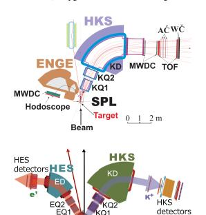
FIG. 1. (Color online) Schematic illustration of the experimental setup, technique, and upgrades for the Hall C HKS hypernuclear spectroscopy experiments E01-011 (top) and E05-115 (bottom).
