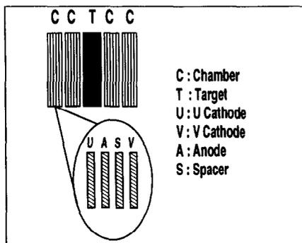
Figure 2. Conceptual design of an ACT segment. Target is inserted between 2 sets of chambers.
