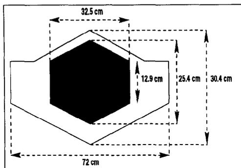
Figure 1. Front view of ACT. The chamber parameters are trimmed to follow the target shape.
