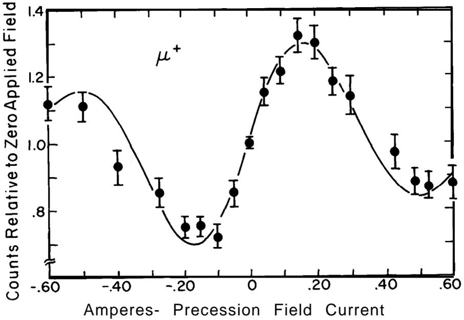
Figure 4. Variation of gated 3-4 counting rate with magnetizing current. The solid curve is computed from an assumed electron angular distribution  $1-1/3 \cos\theta$ , with counter and gate-width resolution folded in.
