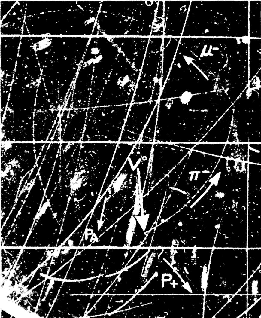
Figure 2. Example of  $K^0_{L1} \rightarrow \pi^+ + \pi^-$  neutral particle.  $P_+$  is shown to be a pion by ionization measurements.  $P_\lambda$  is a proton track used in the ionization calibration.
