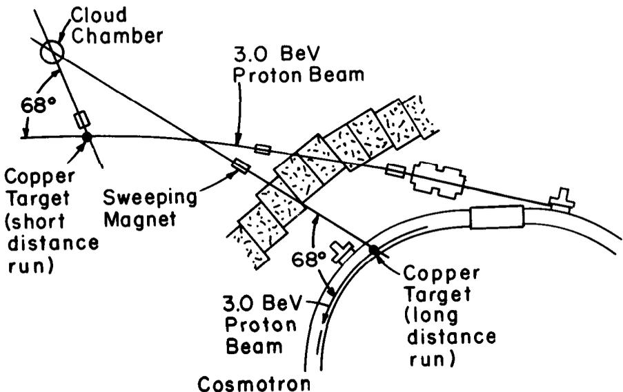
Figure 1. Experimental arrangements for lifetime study.
