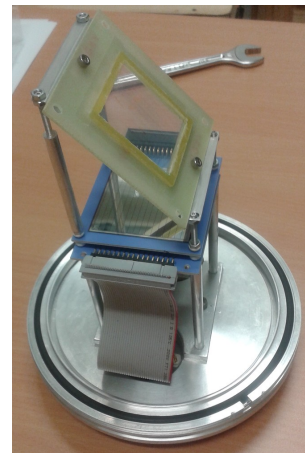
Figure 1: Experimental setup housing the segmented silicon telescope (SITE), originally used for the measurement of the ^7\text{Be}(n, p) reaction.
